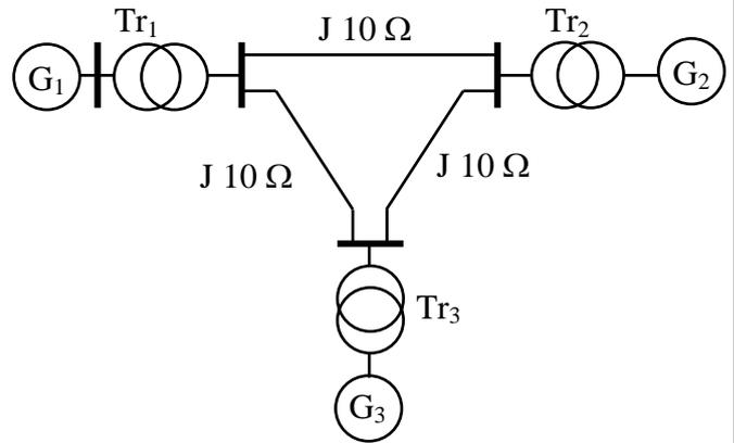
Tr<sub>1</sub>: 20 MVA, 11/110 kV,  $x=J0.12$  p.u.
